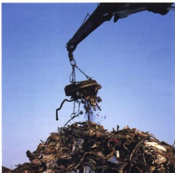
Figure 16.15 An electromagnet in use in a scrap yard
